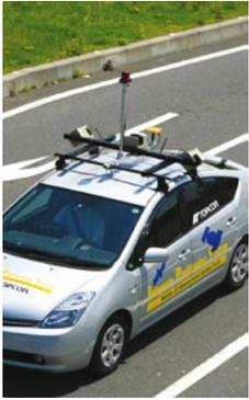
The IP-S2 standard system includes three high-resolution LiDAR scanners that cover the vehicle path at ground level and sweep the adjacent areas to a distance of 30 meters.
