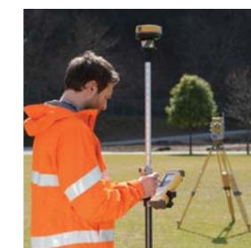
**One-man Survey System - Quick-lock and IR communication technology**
